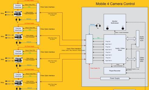
Each block can manage an incoming SDI signal (e.g. a camera), an outgoing SDI signal (e.g. Program) and an intercom audio signal.
